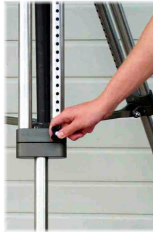
Securing the tripod legs
