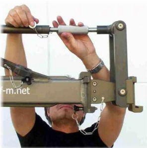
Securing the parallelogram rod
