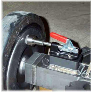
Locked wheel brake on Base Dolly
