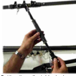
Setting the adjustable rigging rod support
