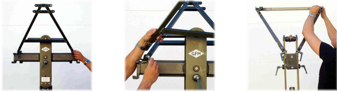
Rigging harness assembly
