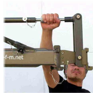
Levelling the angle adjuster
