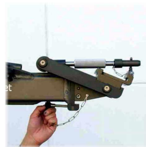
Securing it with a safety pin
