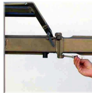
Securing the arm with a safety pin
