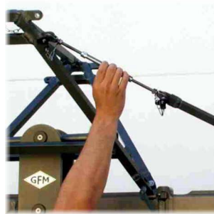
Adjusting the turnbuckle!
