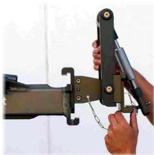
Mounting the angle adjuster
