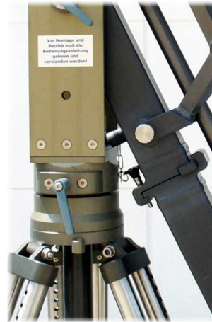
Avoid forceful stops into the pan bearing
