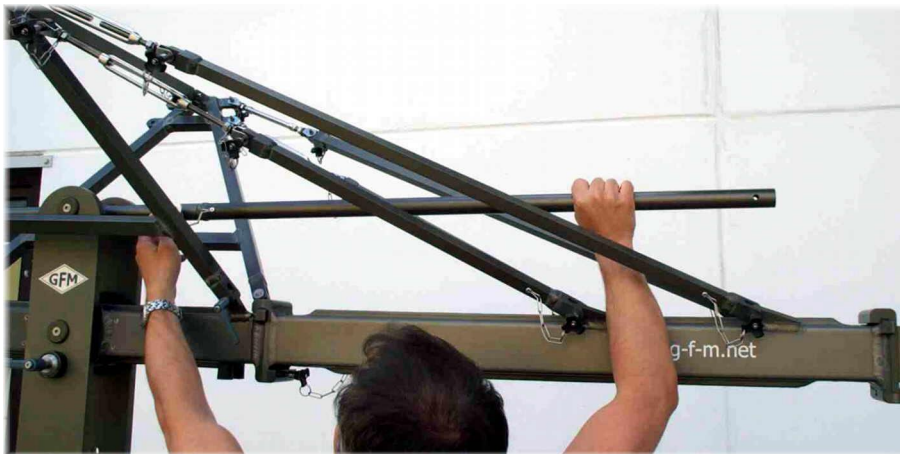
Connecting the parallelogram rod
