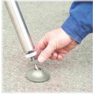
Levelling the tripod
