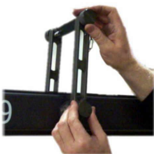
Connecting the parallelogram support
